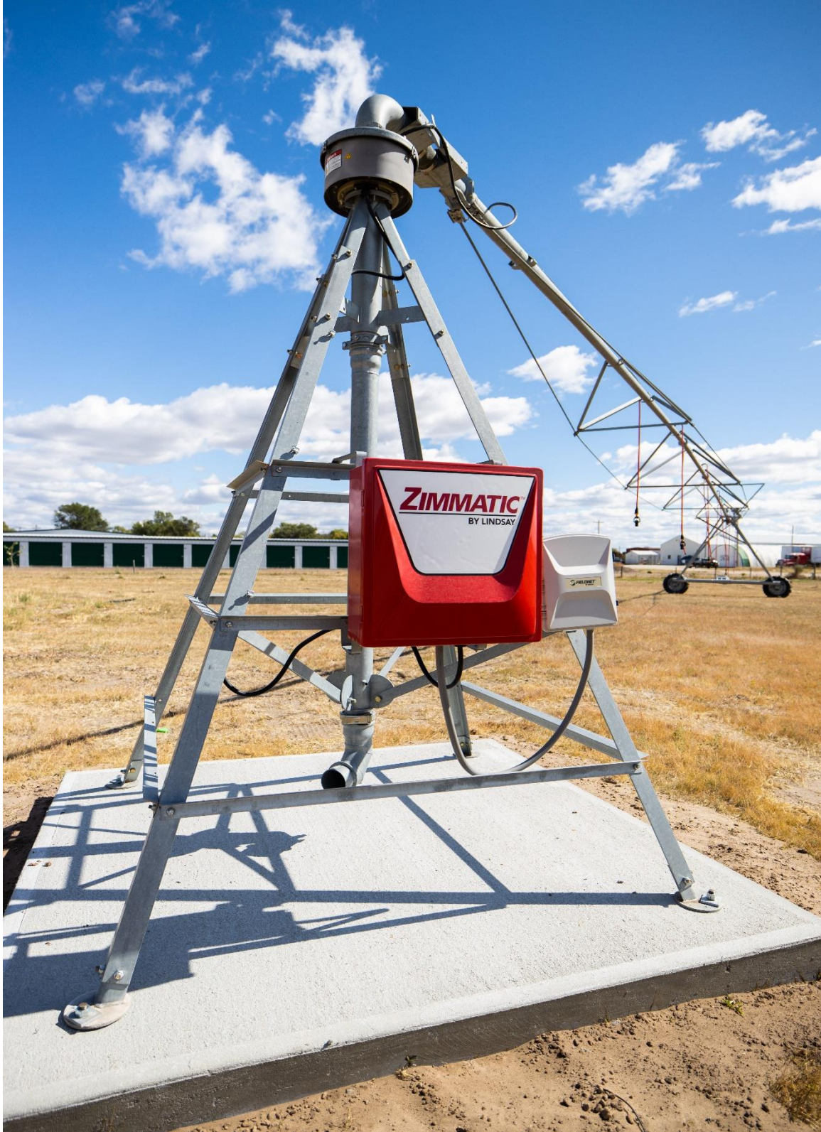
Fully Functional 121' center pivot irrigation system donated by Lindsay -Zimmatic. Set up with the newest FieldNet technology and 7 different sprinkler packages.
